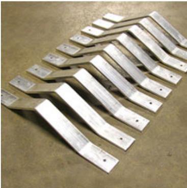
Aluminum Brackets Bent and Punched
