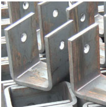
Bent Steel Plates
