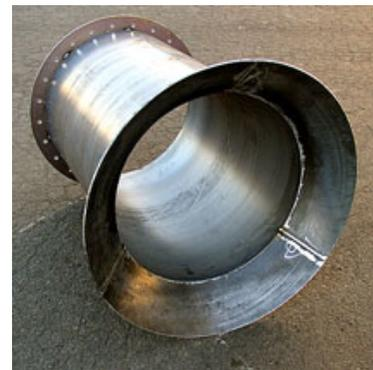
Rolled Cylinder Welded and Punched
