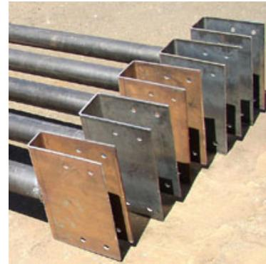
Fabricated Pipe Columns Steel
