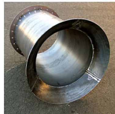
Rolled Cylinder Welded and Punched
