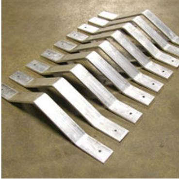
Aluminum Brackets Bent and Punched
