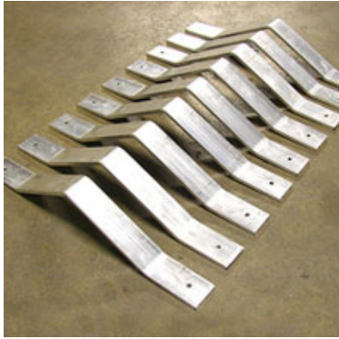
Aluminum Brackets Bent and Punched
