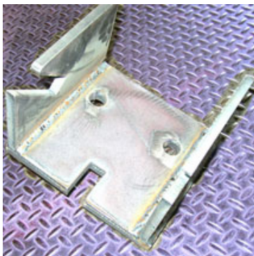
Stick Welded Steel Bracket
